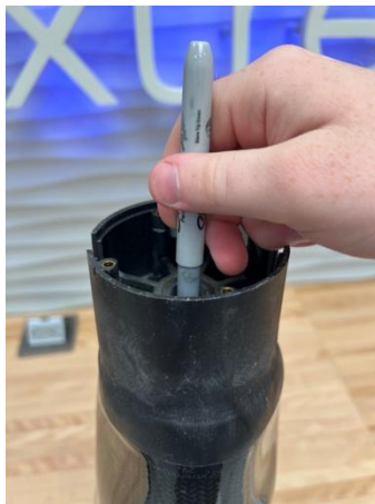
Figure 2: Marking Drilling Location
